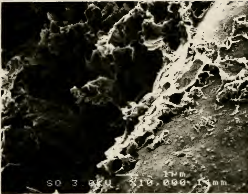
Figure 2.10c SEM photomicrograph of facsimile treated with OH followed by sequential applications of MMA and MTMOS (SQ) and etched with 1M HCl. 3.0KV, 10000X magnification.
